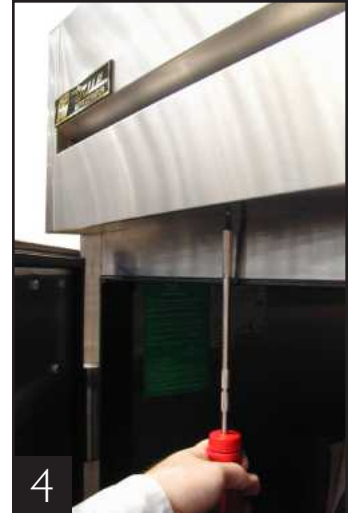
Rainshield removal, bottom screws.
