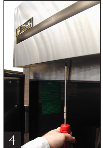
Rainshield removal, bottom screws.
