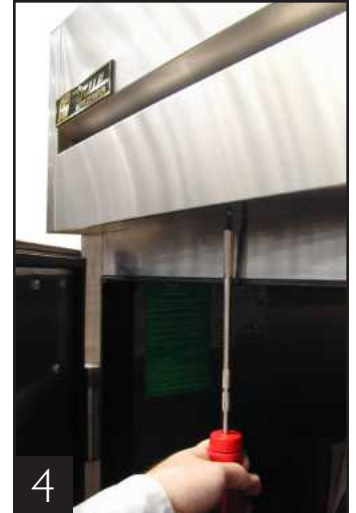
Rainshield removal, bottom screws.
