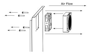
13. Remove and replace fan. Take special care to properly route fan wire.
