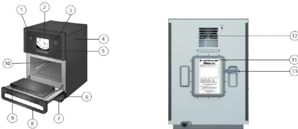
Figure 1.2: e1s front and rear views – parts and safety devices
