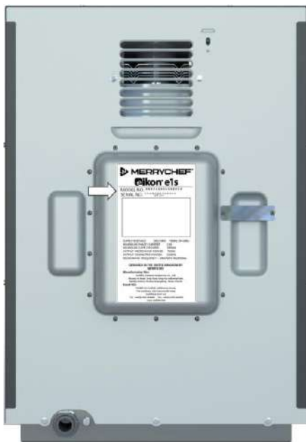
Figure 2.5: e1s rear view with nameplate
