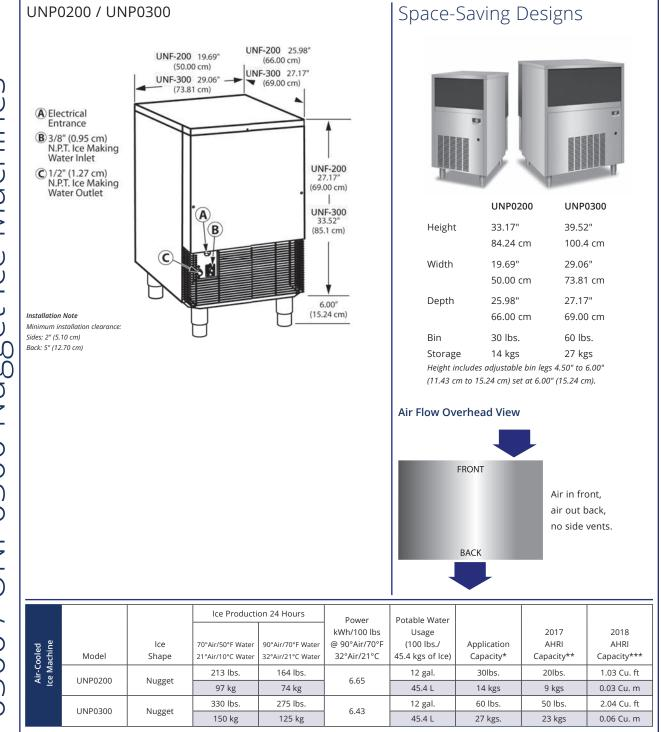
"A" following model number indicates "Air" condensing unit.
