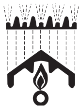
Burner heats radiant which radiates heat to the grate and food.
