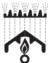
Burner heats radiant which radiates heat to the grate and food item.
