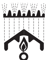
Stainless steel burners and radiant combination creates a searing hot surface temperature.
