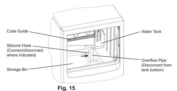
3) Pinch and push down the snaps on both sides of the bracket to unhook the water tank from the square holes, and pull it about 1" towards you.
