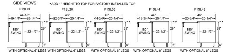
Note: Available with compressor left or right. Compressor left model shown.
