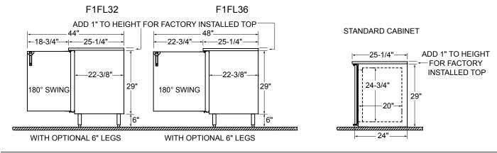
Note: Available with compressor left or right. Compressor left model shown.
