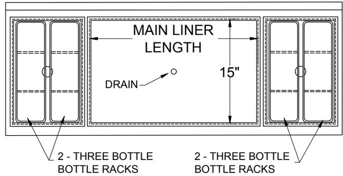
Plan view detailing two bottle well models
