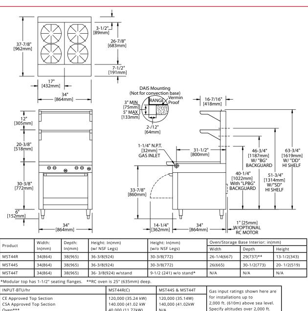
RC=Range w/Convection Oven R=Range w/Oven S=Range w/Storage Base T=Modular Top \*\*\* Oven rated 35,000 BTU (10.25kW) for Propane Gas
