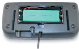
ERS-60 with rechargeable battery option
