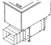
5. Put eight provided screws through the telescoping duct side walls to hold it at the desired depth.
