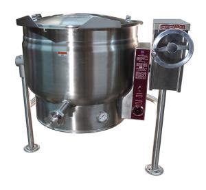
Shall be a Crown Model\_\_\_\_\_\_\_, self-generating, electric tilting full jacket kettle, low height. A double wall kettle interior shall form a steam jacket around the kettle. The jacket enclosure shall contain distilled water which is factory sealed. The bottom of the kettle shall be of hemispherical design for superior heat circulation.
